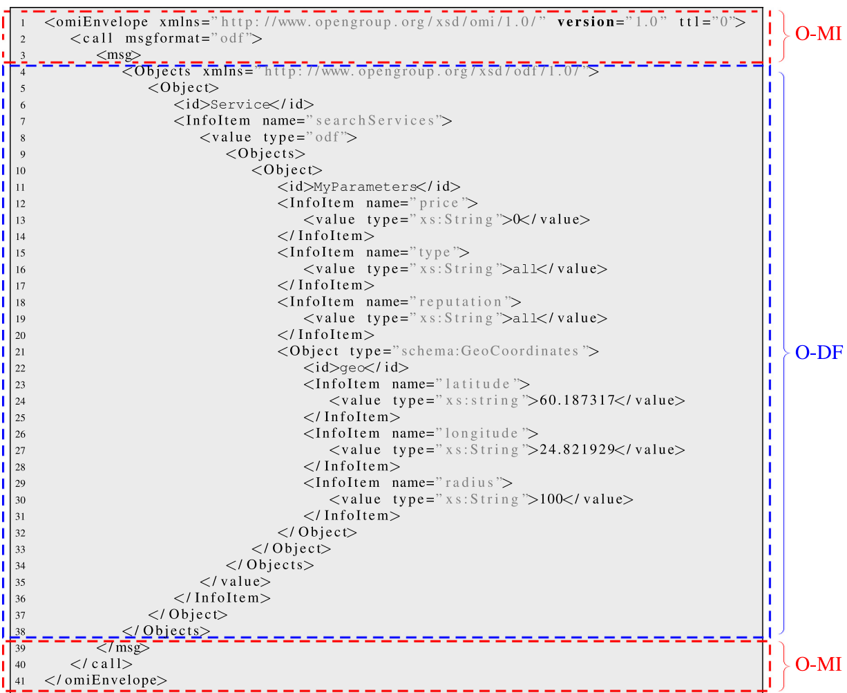
Fig. 8. IoTBnB standardized REST API to request for existing IoT data/services in a given geographical area.
